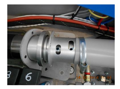
I. Slide subassembly A (16) completely into subassembly B (17).
