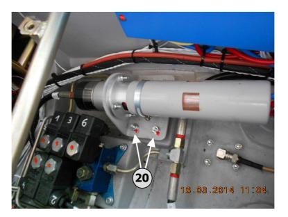
p. Position the pump unit on the four shock-absorbers. Apply medium strength threadlocker (loctite 243) to the M6 thread of
