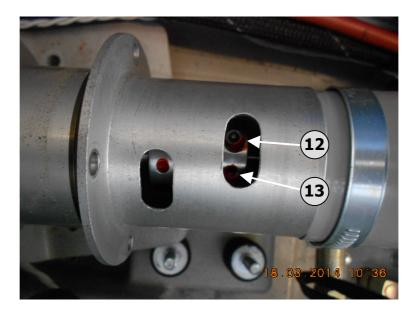
a. Rotate the coupling enclosure and the coupling until the clampscrew M3 x 10 (12) and the stud-screw M4 x 8 (13) can be reached through the rear aperture in the coupling enclosure. In order to achieve this, it may be helpful to use a 2.5 mm Allen wrench as a lever
