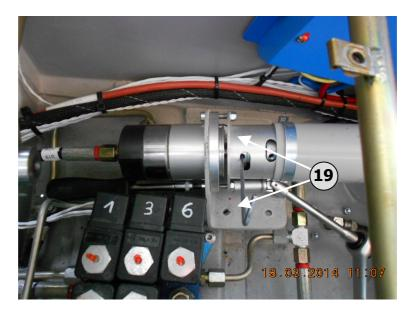
m. Equip the four M5 screws (19) with new locknuts, and use a 4 mm Allen wrench and an 8 mm wrench to lightly screw pump, mount and coupling enclosure together with a small gap between the components.
