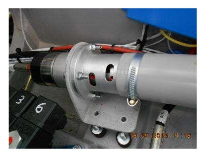
o. Use a 2.5 mm Allen wrench to tighten both stud-screws in subassembly B. Apply inspection lacquer to the screw connections.
