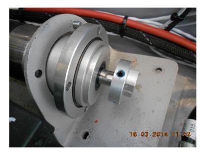
k. Slide the subassembly B (17) so far away from the pump as the notch in the pump shaft allows, and use a 2.5 mm Allen wrench to slightly tighten the M5 x 12 stud-screw.
