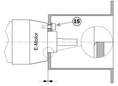
Check whether there is a gap between the motor and the coupling enclosure. If this is the case, then use a 2 mm Allen wrench to remove the four M3 x 8 screws (15), which connect the motor and the coupling enclosure.
