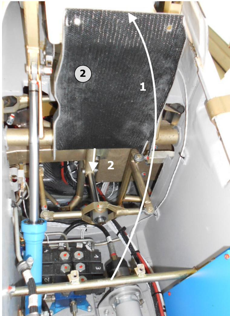
In the cockpit; position the flap control lever in position -3.
