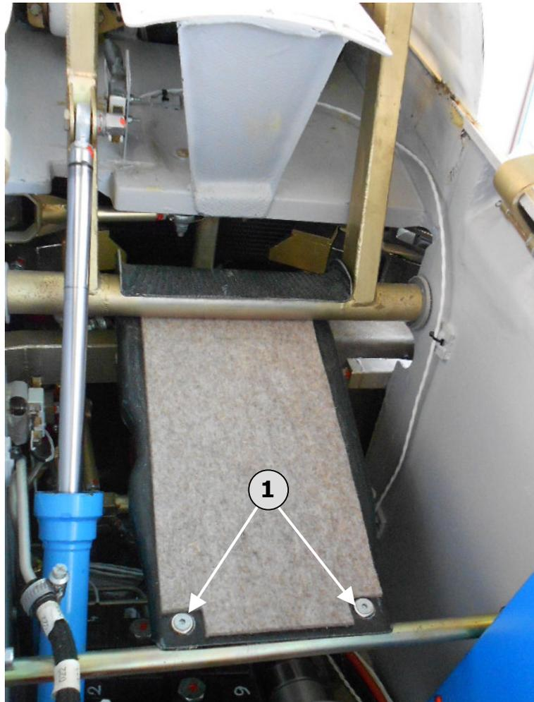
Use a 3 mm Allen wrench to remove the two M5 countersunk screws including collars (1).
