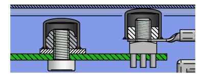
n. Apply Loctite 243 to the five M4 screws that were removed in procedural step 3. 0. Use these to mount the cover to the base-plate.
