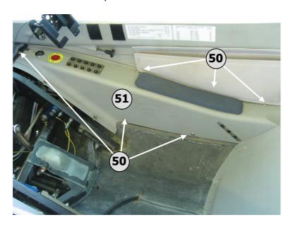
Use a 3 mm Allen wrench to remove the six M5 countersunk screws including collars (50) that are used to mount the side panel (51). Put the screws aside. Remove the side panel.
