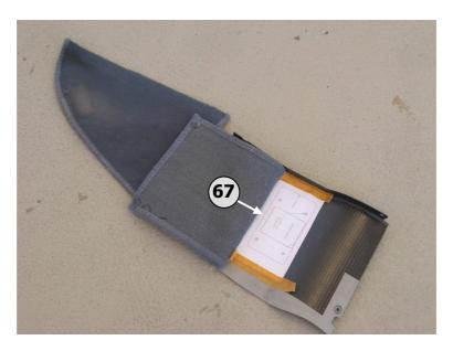
Remove the lower leg-rest from the aircraft and use tape to position the attached cutout-mask (67) so that the following criteria are fulfilled:
