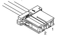
Remove the cable (14) from plug-in position 1: Insert a small slotted screwdriver into the connector housing and press the securing latch down and away from the connector. While doing so, gently pull the connector out of the connector housing. Remove the remaining connector housing and cable (these parts were installed as a part of TM 904-2 level 1).
