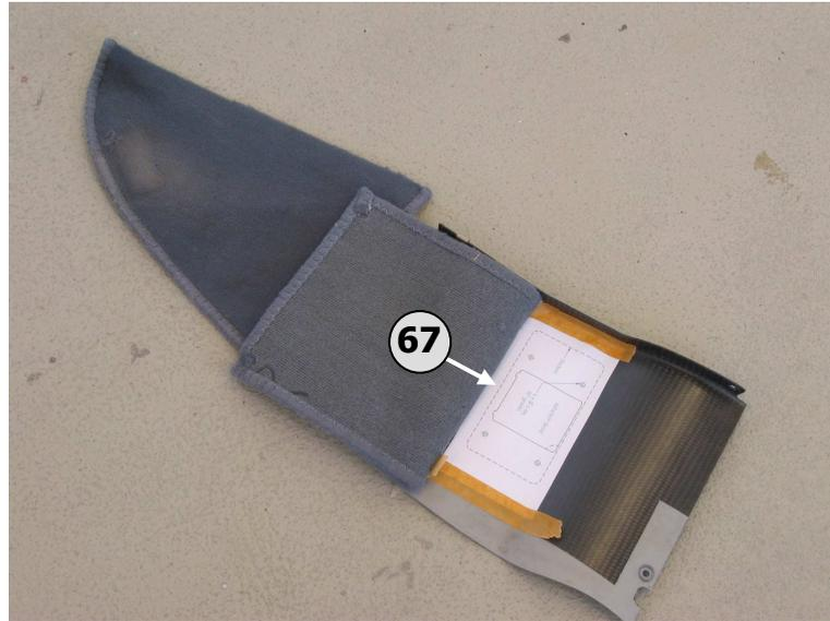
Remove the lower leg-rest from the aircraft and use tape to position the attached cutout-mask (67) so that the following criteria are fulfilled:
