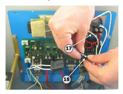
Follow the switching cable (17) to the inline connector (18), and disconnect said connector. If the connector is covered by heat shrink tube, then remove this tube before proceeding to disconnect. Some aircraft have the connector directly on the DC/DC converter PCB. If this is the case, then disconnect the cable here.
