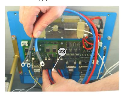
Remove the 12V supply connector (23) from the socket on the HMM PCB (leftmost black socket in picture). To release the connector press both securing latches together and keep them pressed while connector housing is pulled out of the socket.
