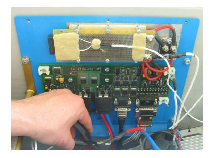
Use a pair of side cutting pliers to cut open and remove the cable-ties holding the cable bundle passing underneath the HMM together. The DC/DC converter is now electrically completely disconnected from the rest of the system.
