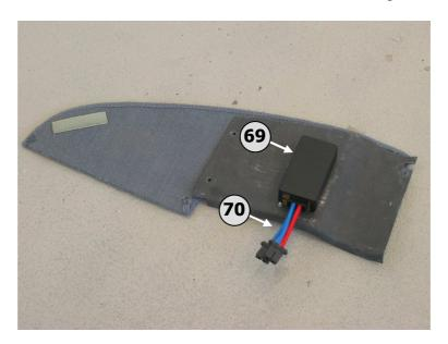
Position the new maintenance socket (69) underneath the lower leg-rest. Make sure that the cover opens and closes easily. Apply Loctite 243 to the four M4 countersunk screws, and then use an Allen wrench to attach the maintenance socket to the lower leg-rest. Apply inspection lacquer to the screws.
