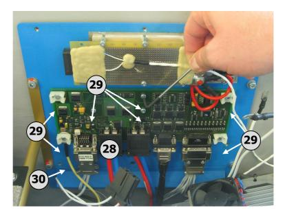
Re-insert the 12V supply connector (28) into the socket on the HMM PCB. Make sure that the securing latches engage the socket so that the connector can no longer be pulled out of the socket.
