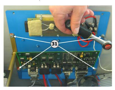
Use a 5 mm allen wrench to remove the four M6-Screws (31) that fix the base-plate to the motor-bay wall.
