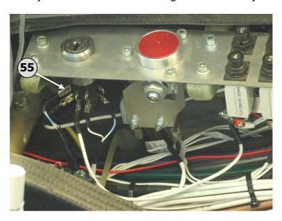
Fold the cable lug with the white wire back along the main cable and insulate it as follows: Slide one of the two 5 cm heat shrink tubes, (found in the TN kit) over the cable so that said cable lug is fully covered, and use a hot air gun to shrink the tube. Install the remaining cable lug with the blue striped wire (55) on key-switch terminal (S1).
