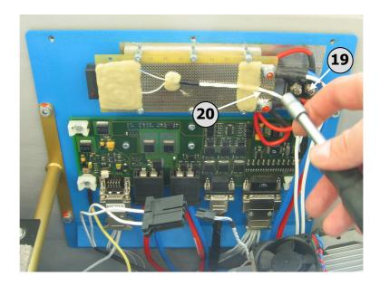
Use a 7mm wrench or socket to disconnect the minus cables (19) from the topmost terminal on the DC/DC converter PCB (20). If the white cable is unmarked or not clearly marked, mark the cable to indicate minus using a black or blue permanent marker.
