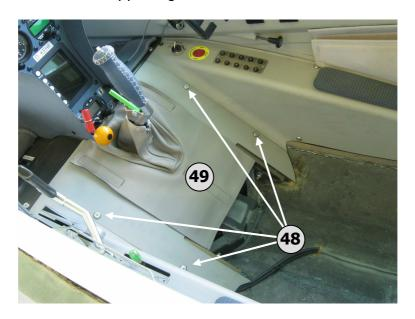
Use a 3 mm Allen wrench to remove the four M5 countersunk screws including collars (48) that are used to mount the upper leg-rest (49). Put the screws aside. Remove the upper leg-rest as well as the leather stick-cover.
