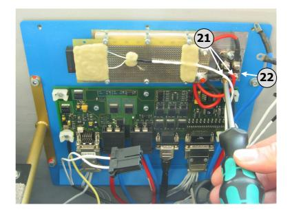
Use a Philips-head screwdriver to disconnect the 12V cables
