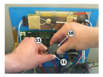
Remove the inline fuse (10) installed as a part of TN 904-2 level 1. To release the connector press both securing latches (11) together and keep them pressed while connector housing is pulled out of the socket.
