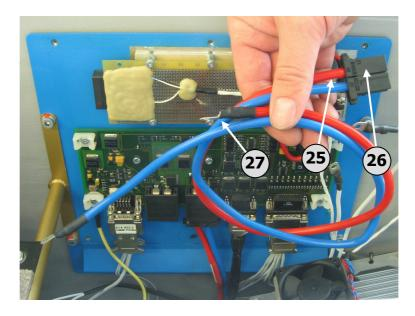
Insert the new red cable found in the TN-kit (25) into the now free plug-in position 1 (26). Make sure that the securing latch engages the connector so that it can no longer be pulled out of the connector housing.
