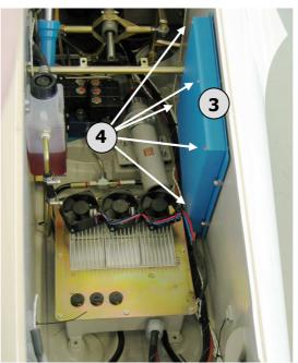
The DC-DC converter and the HMM share a common housing (3) located at the right engine bay wall. In this procedural step the cover is removed from the common housing.
