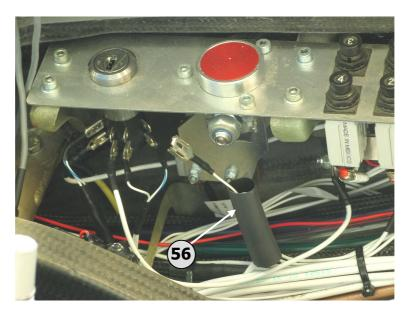
Fold the cable lug with the with the blue striped wire back along the main cable. Slide the second 5 cm heat shrink tube (56) over the cable so that said cable lug is fully covered, and use a hot air gun to shrink the tube.
