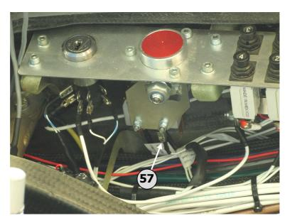
Install the remaining cable lug (57) with the white wire on emergency-off switch terminal (N2). Pull lightly on the cable lug to check for proper locking.
