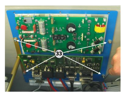
Slide the new base-plate with DC/DC converter into position between motor-bay wall and the transverse shaft of the propeller blade catcher.
