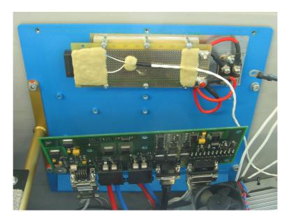
The HMM PCB has now been completely separated from the base-plate and the DC/DC converter.
