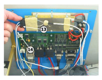
Disconnect the supply connector (13). To release the connector press both securing latches together and keep them pressed while connector housing is pulled out of the socket.
