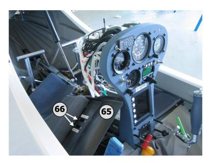
Tilt the lower leg-rest (65) so that it's underside becomes accessible for further work.
