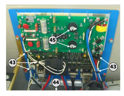
Use the cable ties (43) from the TN kit to fix the cable routing as shown in the picture above. Also use cable ties to fix the cable bundle (44) that was loosened in procedural step 4.k.
