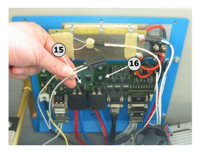
Insert this free connector (15) into the now free plug-in position 1 (16). Make sure that the securing latch of the connector engages so that it can no longer be pulled out of the connector housing. This completes removal of parts installed as a part of TM 904-2 level 1.
