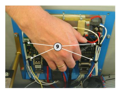
Remove the 4 cable ties (9) a pair of side-cutting pliers.
