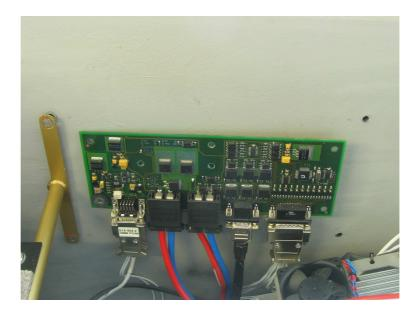
Remove the base-plate including the old DC/DC converter.
