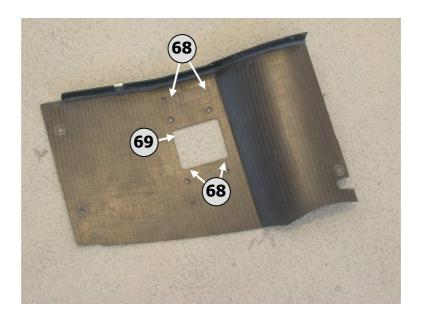
Drill and countersink the four  $\varnothing$  4.3 mm holes (68). If required, then remove the carpet first..
