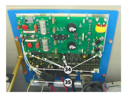
Apply Loctite 243 to the seven M4 screws that were removed in procedural step 4. p (34). Use these to mount the HMM-PCB to the base-plate.
