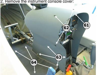
2. Remove the instrument console cover:
