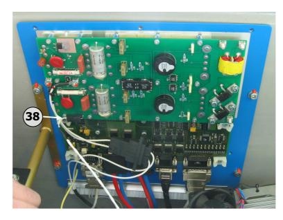
Connect the switching cable (38) that was disconnected in procedural step (4.h) to the fitting socket on the DC/DC converter PCB. Make sure that the securing latch engages the socket so that the connector can no longer be pulled out of the socket.
