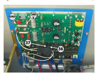
Insert the 288V connector that was disconnected in procedural step 4.d into the 288V adapter-socket (37), which hangs down from the DC/DC converter PCB. Make sure that the securing latches engage the socket so that the connector can no longer be pulled out of the socket.
