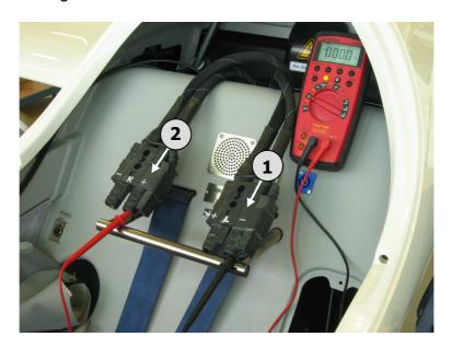
Use a Voltmeter to measure the voltage between the minus connector (1) of the left wing connector and the plus connector (2) of the right wing connector. Set the voltmeter to measure DC voltages at a 300V range. Take note not to measure against the bridging cable, which connects the right wing connector with the left wing connector. The measured voltage should not be above 2 V. Should a higher voltage be measured, then contact Lange Aviation GmbH.
