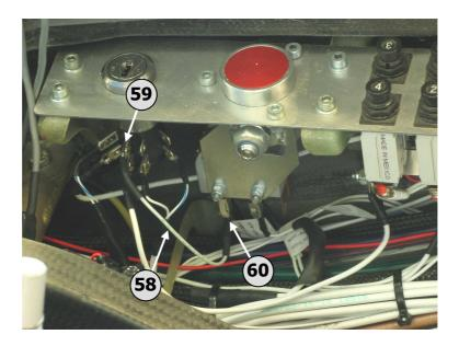
locate the white bridge-cable (58) in the TN kit, and use it to connect key-switch terminal (S2) with emergency-off switch
