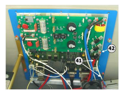
Connect the minus cables (41) that were disconnected in procedural step 4. j to the two top right terminals (42) on the DC/DC converter PCB as shown on the picture above. Apply Loctite 243 (blue) to the M4 nuts before installing them, and use a 7mm wrench or socket. Be careful not to apply too much torque or pressure, as this can lead to the thread of the terminals to shear off or damage to the PCB. Apply inspection lacquer to the nuts.
