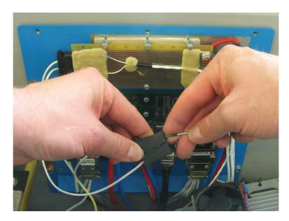
Unplug both connectors from the connector housing that was disconnected in procedural step 4.b. To unplug the connector from the housing, insert a small slotted screwdriver into the connector housing and press the securing latch down and away from the connector (see sketch). While doing so, gently pull the connector out of the connector housing.
