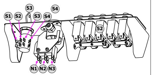
Next to the circuit breakers (52), the now accessible circuit breaker panel also contains the key-switch (53) and the emergency-off switch (54). Now remove the two cable lugs
