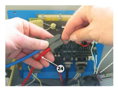
Remove the red 12V cable form the 12V supply connector.
